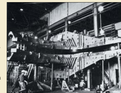
The first sector of the TRIUMF cyclotron magnet assembled at the manufacturer's (Davie Shipbuilding Limited, Quebec) prior to dispatch to the site at the University of British Columbia.
